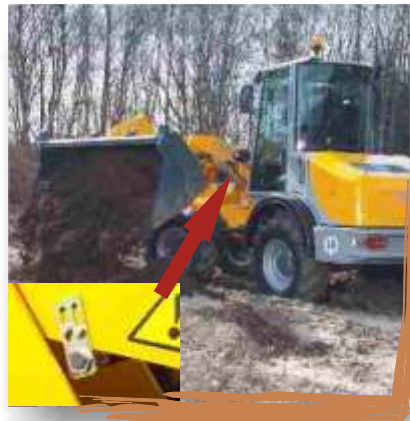
Lowering cut-off automatics avoids damage to the tires in swivelled position
