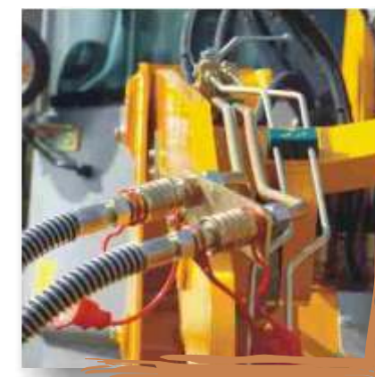
Additional connection for hydraulic attachments, e.g. concrete-mixing bucket or power sweeper
