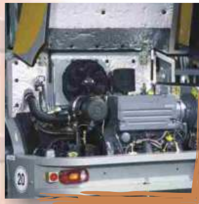
Extremely good accessibility for inspection and maintenance works due to the GFK engine cover that can be opened widely
