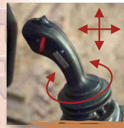
Electro-hydraulic anticipatory control via multifunctional joystick; swivelling function by turning the joystick
