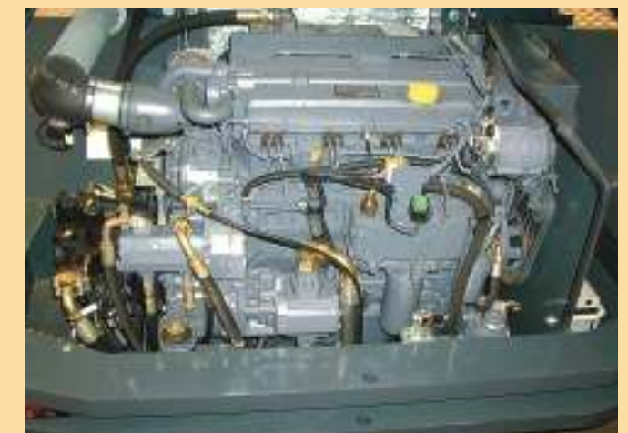
The PAUS-Telescopic loader RL 1252 SL-B gets its performance from the 4-cylinder-Deutz-Diesel engine with 93 kW/126 hp which is water-cooled and poor of noise with merely 2.300 rpm. The engine meets emission limiting values being far below the limits of the valid Euro-norms.
