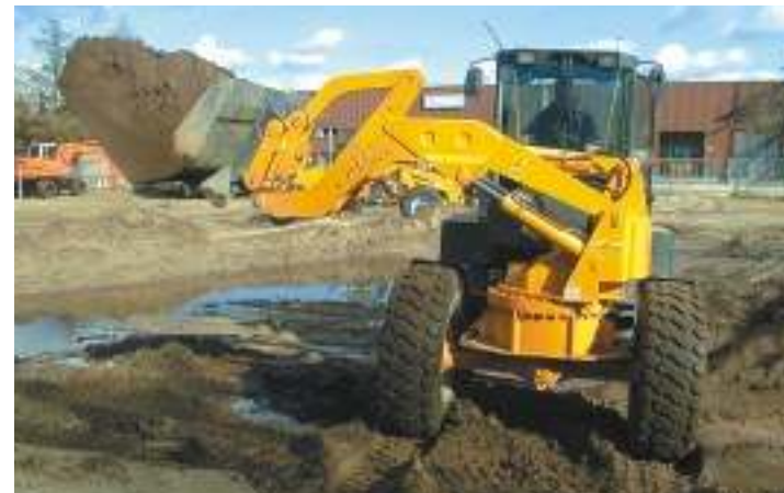
Swiveling device with two directly articulated cylinders for constantly backlash-free working with maximum operating security.
