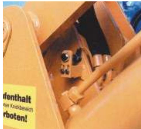
The lowering cut-off automatics avoids uncontrolled damages on tires during swiveling position.
